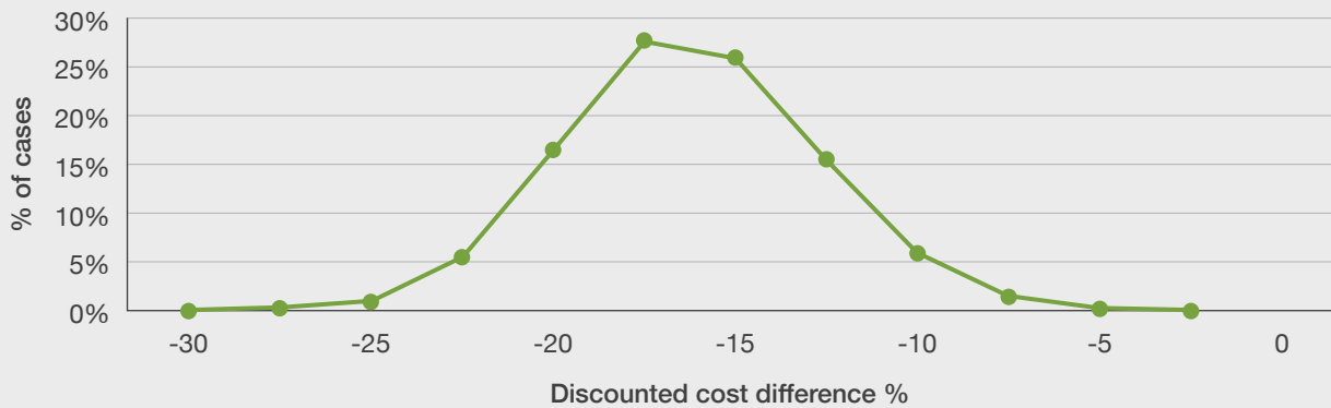
Figure 1: Distribution of discounted total discounted cost: concrete v asphalt pavement (6% discount rate, 40-year horizon)
