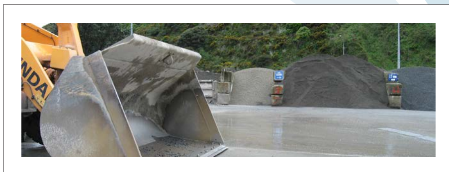
Figure 9: Aggregate storage in stockpiles at a loader-fed concrete plant
