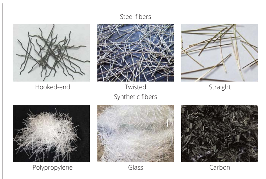
Figure 10: Range of structural and non-structural fibres used in concrete
