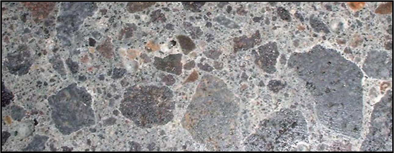
Figure 9: Concrete containing New Plymouth aggregates
