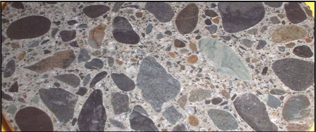
Figure 17: Concrete containing Kaikoura aggregates
