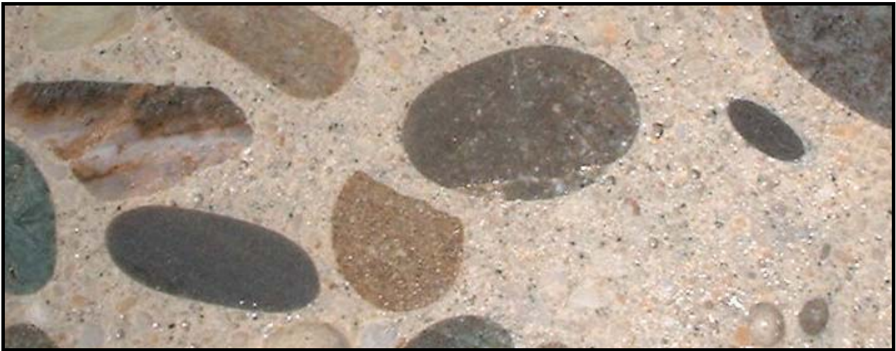
Figure 22: Concrete containing Oamaru aggregates
