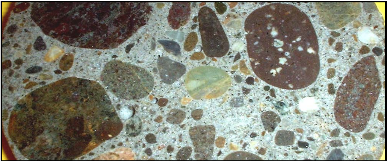
Figure 26: Concrete containing Invercargill aggregates
