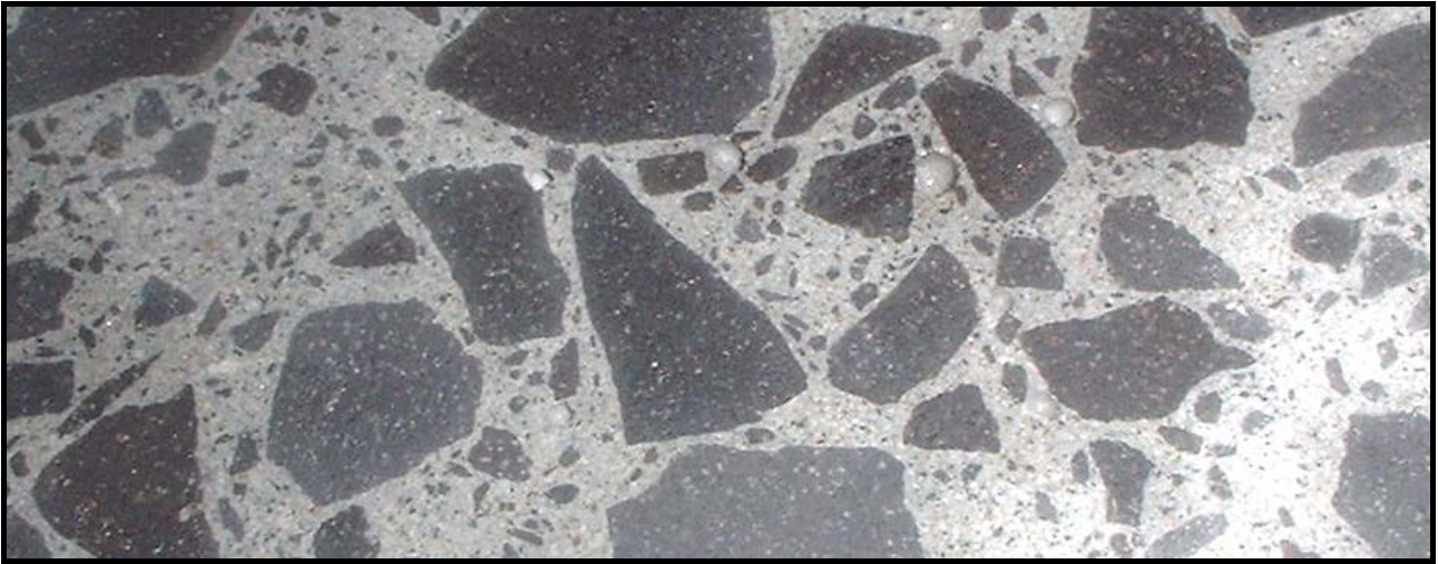
Figure 5: Concrete containing Pukekawa aggregates
